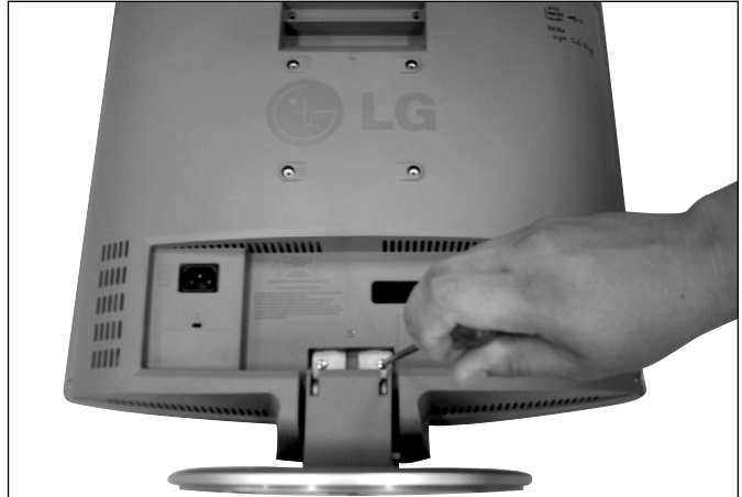
#2 Detached stand assy (Remove the screws)
